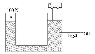
Figure 2 above shows a hydraulic machine.
